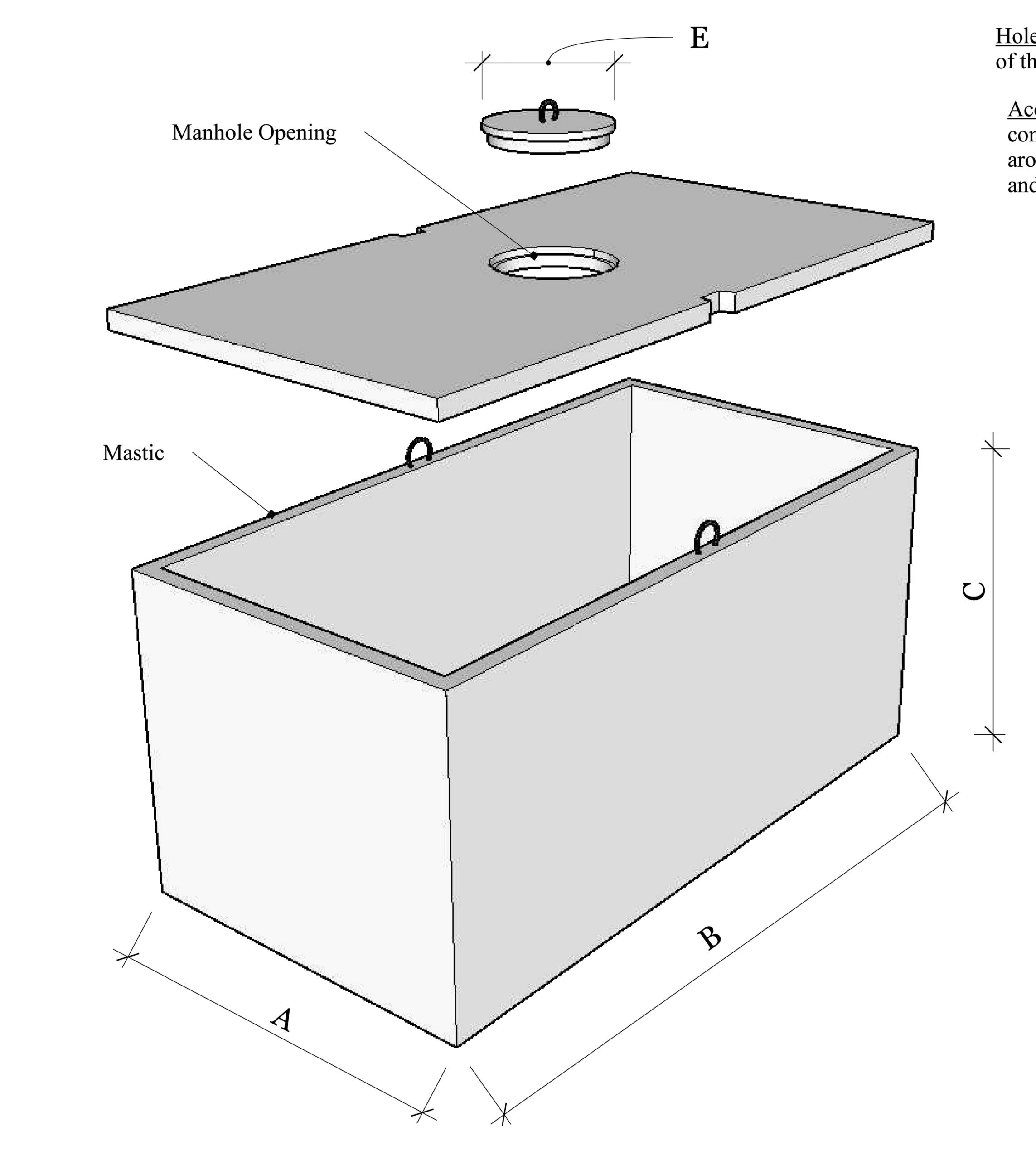
Hole Dimensions: The hole should be dug 2' wider and 2' longer than the external dimensions of the tank. The bottom should be leveled with 4" of graded material in the bottom.
